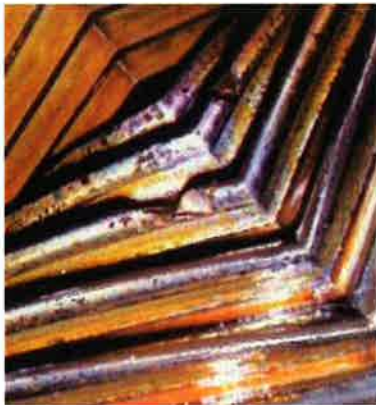
WCA CALENDAR GEARBOX CONDITION PRIOR TO CASTROL – HEAVY WEAR AND MISSING TEETH FRAGMENTS
